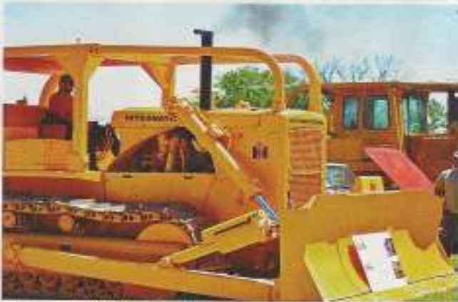
Blowing out a bit of smoke, the operator is revving the IH built DT-817 diesel engine. One advantage over the TD-24 is the 817 engine is direct start on diesel, while the older machine started on gasoline then switched over to diesel. The 24 volt starting model used power from four 6 volt batteries. The batteries were kept charged by a 15 amp alternator.
