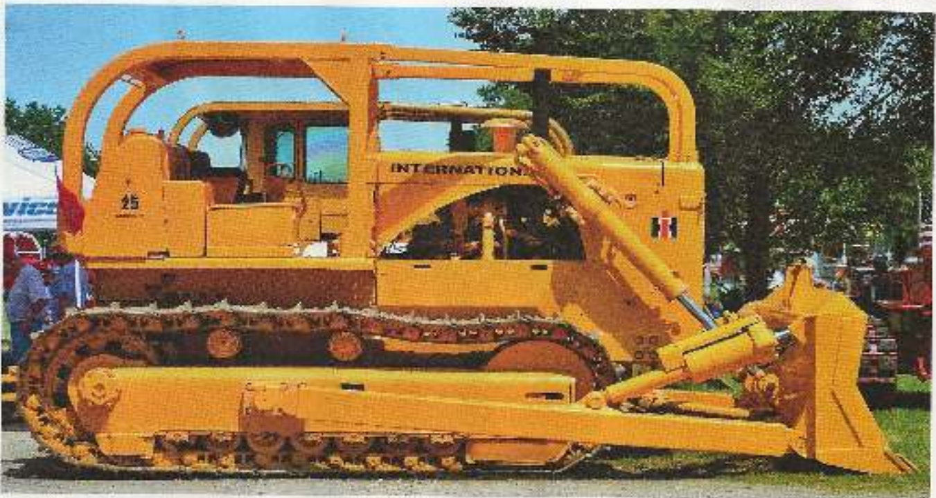
There are 48 shoes on each track, providing 5,662 sq. inches of ground contact with 24 inch wide shoes. The tractor, without the blade, is 137 inches long. Differential steering provides full power to both tracks during turns.
