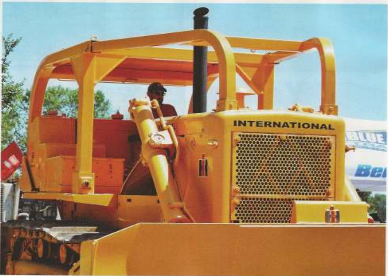
Looking closely, you can see the operator seating on the big TD-25. You notice that the operator's floor is level with the top of track fenders providing easier entry and exit plus a wide platform to stretch out your legs.
